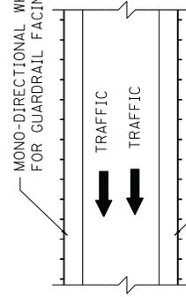
MONO-DIRECTIONAL WHITE DELINEATOR FOR GUARDRAIL FACING TRAFFIC
